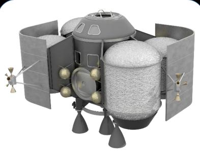
Mars Ascent Vehicle (MAV) is a launch vehicle landed on Mars to put crew back into orbit.
